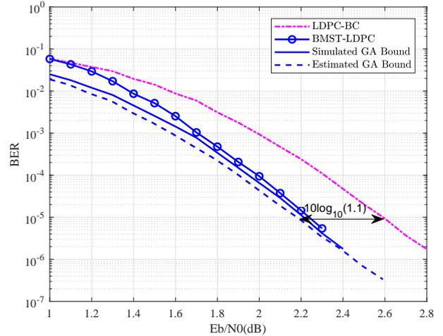
Fig. 2. BER performance and the GA bounds of the BMST-LDPC codes. The basic code is a rate  $1/2$  (3,6)-regular LDPC-BC with length 1024. The superposition fraction for encoding is  $\alpha = 0.1$ , and the decoding window size is  $d = 3$ .
