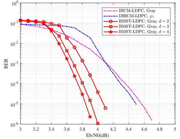
Fig. 5. BER performance of the BMST-LDPC codes with 16-QAM constellation. The basic code is a rate 1/2 (3,6)-regular LDPC-BC with length 2304. The superposition fraction for encoding is  $\alpha = 0.3$ , and the decoding window sizes are  $d = 2, 3$  and 4, respectively.
