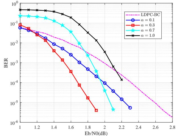
Fig. 3. BER performance of the BMST-LDPC codes with different  $\alpha$ . The basic code is a rate  $1/2$  (3,6)-regular LDPC-BC with length 1024. The decoding window size is  $d = 3$ .
