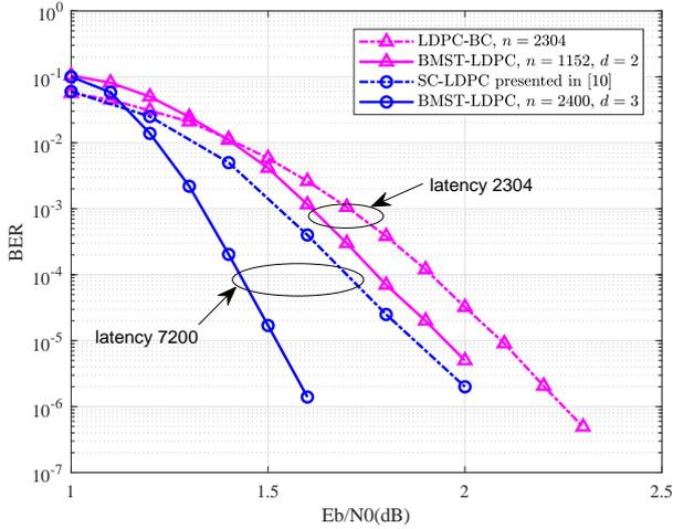
Fig. 4. BER performance of the BMST-LDPC codes, LDPC-BC and an SC-LDPC code [10]. The basic codes are rate 1/2 (3,6)-regular LDPC-BCs with length 1152 and 2400. The superposition fraction for encoding is  $\alpha = 0.3$ , and the decoding window sizes are  $d = 2, 3$ .
