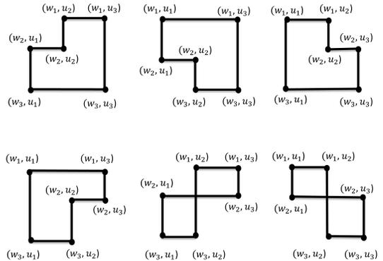
Fig. 1. Patterns of length six cycles in the parity-check matrix.
