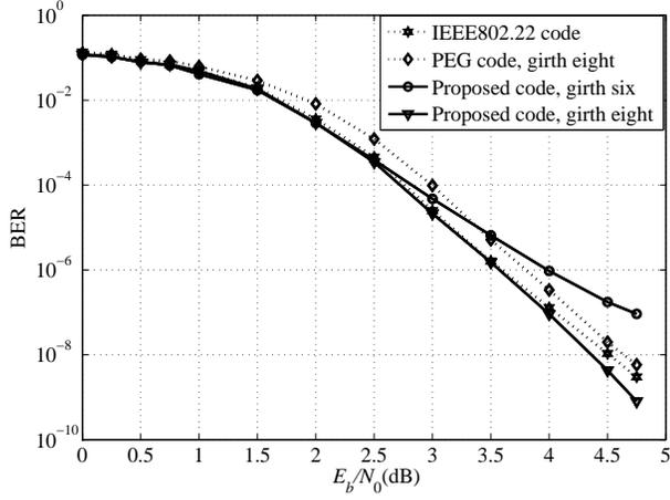
Fig. 2. Performance of the HM-QC-LDPC codes of length 378 bits.
