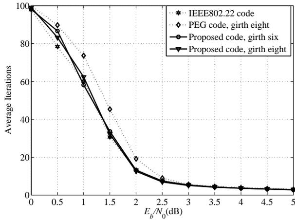
Fig. 3. Average number iterations of the HM-QC-LDPC codes of length 378 bits with the maximum iteration number of 100.
