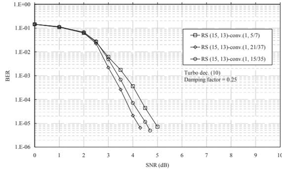
Fig. 3. Turbo decoding performance of the RS (15, 13)-conv. concatenated codes with Gray labelling 16QAM over the AWGN channel.
