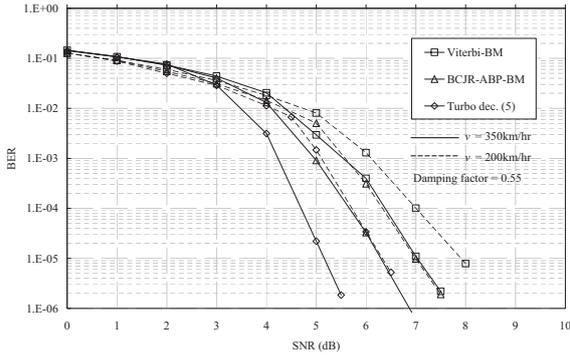
Fig. 7. Turbo decoding performance of the RS (63, 55)-conv.(1, 21/37)<sub>8</sub> code with Gray labelling 64QAM over Rayleigh fading channels.
