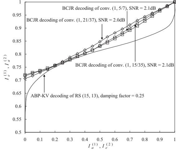
Fig. 2. EXIT performance of the RS (15, 13)-conv. concatenated codes. Gray labelling 16QAM is utilized for transmission over the AWGN channel.
