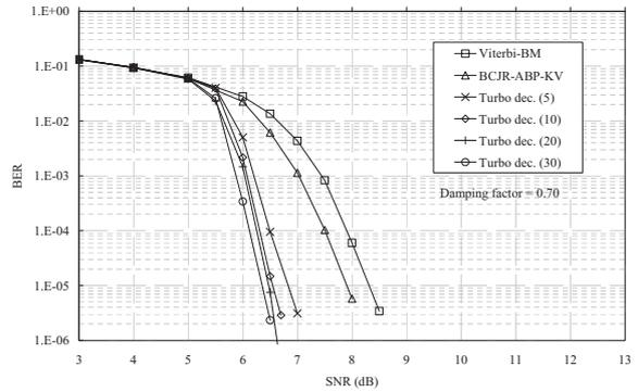
Fig. 6. Turbo decoding performance of the RS (63, 55)-conv.(1,21/37)<sub>8</sub> code with Gray labelling 64QAM over the AWGN channel.
