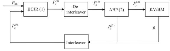
Fig. 1. Turbo decoding block diagram.
