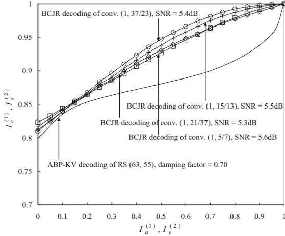
Fig. 4. EXIT performance of the RS (63, 55)-conv. concatenated codes. Gray labelling 64QAM is utilized for transmission over the AWGN channel.
