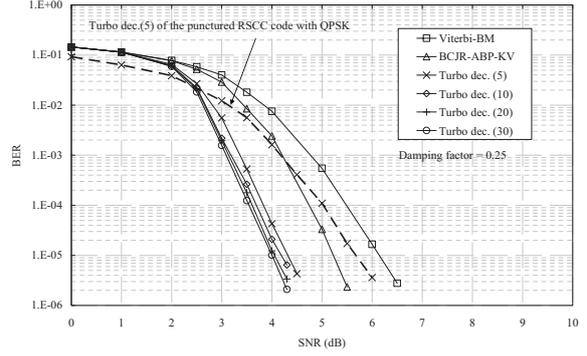
Fig. 5. Turbo decoding performance of the RS (15, 13)-conv.(1,21/37)<sub>8</sub> code with Gray labelling 16QAM over the AWGN channel.
